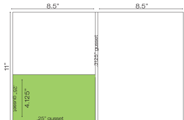
WCP-107 8.5" x 11" Pocket Folder with one taped 4.125" pocket .3125" gusset in center and .25" in pockets (Business Card Slits Optional)
